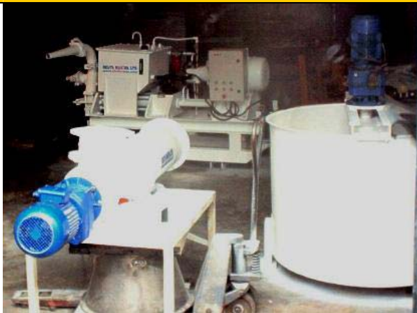
DELTA 3-30 m 3 /hr grout pumps
