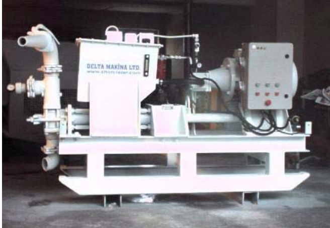
DELTA 3-30 m 3 /hr grout pumps
